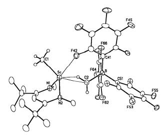
*Figure 1.* Molecular structure of ion pair **3**; aryl groups have been removed for clarity. Selected bond distances (Å): Sc-N(1), 2.060(5); Sc-N(2), 2.093(5); Sc-C(1), 2.221(5); Sc-C(2), 2.703(6); Sc-F(42), 2.390(4); B-C(2), 1.643(9). Selected bond angles (deg): N(1)-Sc-N(2), 95.06(19); Sc-C(2)-B, 138.72(18); Sc-F(42)-C(42), 153.7(4).
