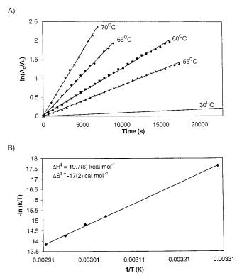
**Figure 9.** (A) First-order kinetic plots for the metalation of **6b** to produce **13b** and SiMe<sub>4</sub> at various temperatures. The complete data set for the run at 30 °C is not shown in the figure; this run took over 80 000 s to go to 5 half-lives. (B) Eyring plot of the temperature dependence of the rate constants.
